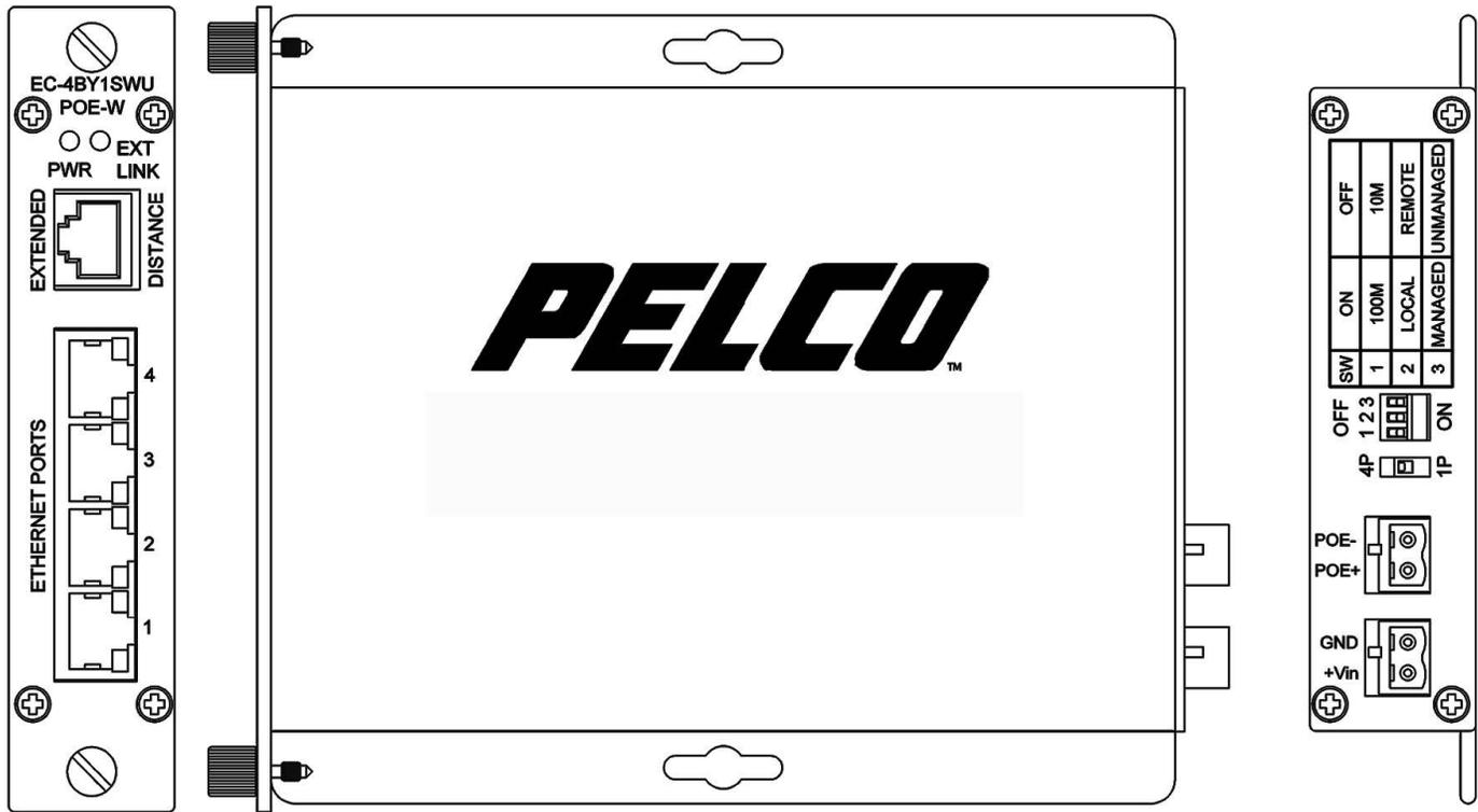
UNIDAD COAX DE MONTAJE EN BASTIDOR O SUPERFICIE (EC-4BY1SWCPOE-W)
